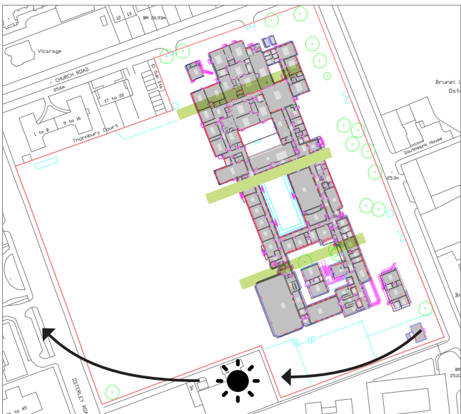
External shading and cross ventilation via courtyards and streets
